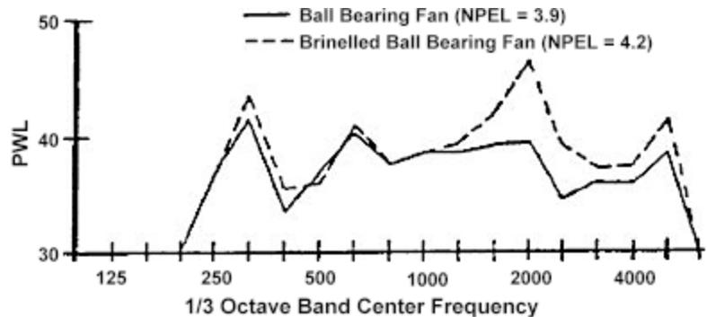
Figure 3: Fan Noise Due to Damaged Ball Bearing
