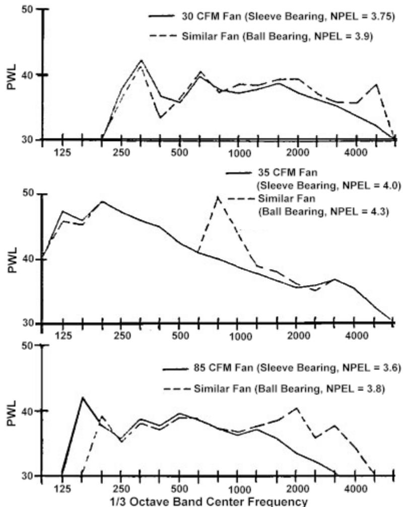
Figure 2: Sleeve Bearing vs Ball Bearing Fan Noise
