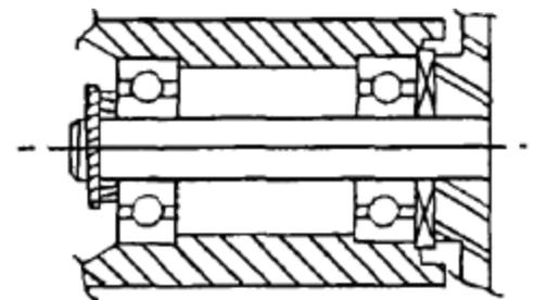
Figure 1-B Ball Bearing Assembly
