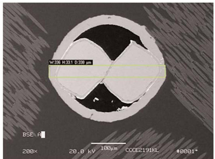
Figure 7: MAP connectors meet or exceed corresponding EIA and IEC radial hole distortion and remaining wall thickness requirements. The images (L & R) show x-axis and y-axis diameter differences of just 27 \mu\text{m} . The left-hand image also shows the minimum wall thickness to be 141 \mu\text{m} .
