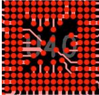
Figure 2 - Example of Via-In-Pad Use for Escape Routing of a MachXO PLD in a 8x8 Mm, 0.5 Mm Pitch, 132-Ball CsBGA Package (LCMXO640-M132/MN132)
