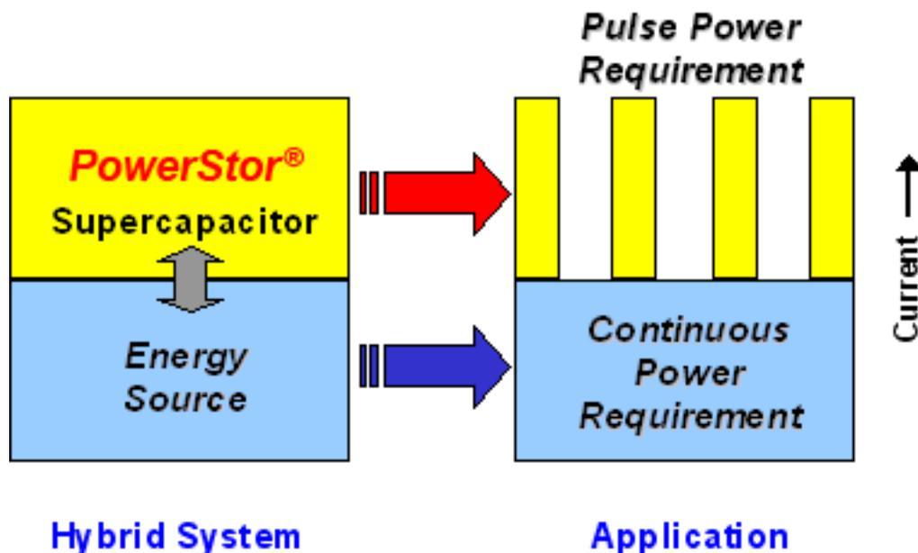
Figure 1 – Hybrid Battery-Capacitor Configuration
