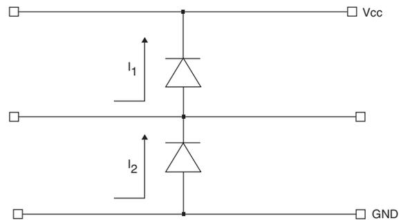
**Figure 2 – Rail to Rail Diode Connection**
